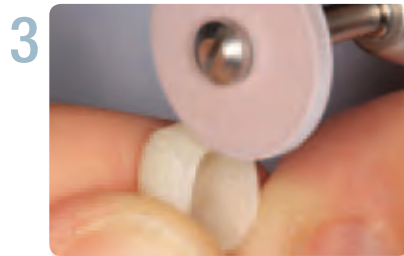
Finish sprue area with medium rubber wheel or cup.
